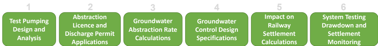
Figure 3: Sequence of steps developed as part of the groundwater management strategy for the works.
