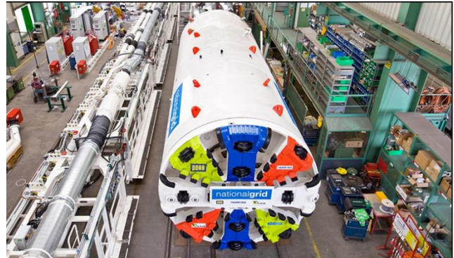
Figure 2. Tunnel boring machine used to construct the Feeder 9 gas pipeline.
